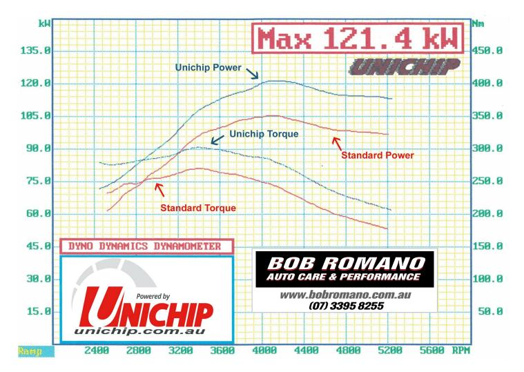
Torque Results: From 264 nm at the wheels. To 305nm at the wheels.
